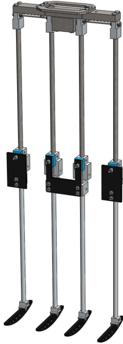
Figure 4.14: The Solid Works drawing the physical walker. This is taken from [10]
